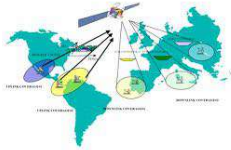
Figure 5.52: AMERHIS full multi-beam cross connectivity
